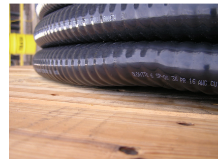
Forklift damage to armored cable.
